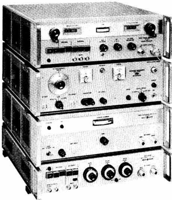
Figure 1. This hp signal generator system provides a 1 watt output with amplitude or pulse modulation. Frequency stability is 1 \times 10^{-5} /sec, 1 \times 10^{-6} /week; PRF's to 1 mc, 20 nsec rise and fall time.
