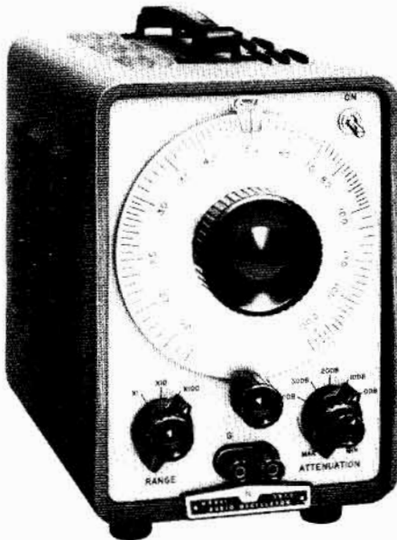
hp 201C Audio Oscillator High Power, 20 CPS to 20 KC
